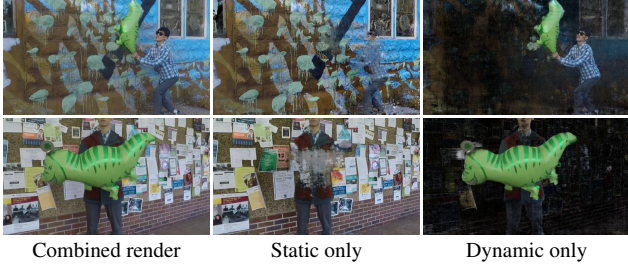
Figure 5: Dynamic and static components. Our method learns static and dynamic components in the combined representation. Note person is almost still in the bottom example.
